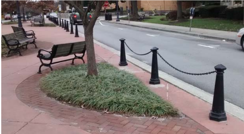
R-7542 DECORATIVE BOLLARD ALONG LAUREL AVENUE MEDIAN, CONNECTED WITH CHAINGS ALONG TREE BOXES TO PROTECT PLANTINGS.
